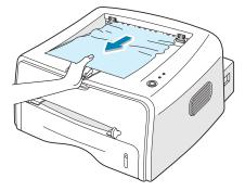
When you pull the jammed paper, if there is resistance and the paper does not move immediately, stop pulling. Continue with the next step. 2 Open the rear output tray.
